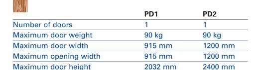
The pocket door kit enables you to create a door that slides into a cavity wall when it is opened. Thus saving valuable space. You can also join 2 kits with a jointing kit (supplied separately) to create a double door opening. Kits come complete with cavity forming studs plus the sliding door hardware and comprehensive instructions. Available in 2 sizes as shown above. For a pair of co-ordinating bi-parting doors, please contact our sales office.
